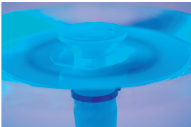
FIGURE 3 THE NEW DESIGN OF DRAIN PORT IN THE CLOSED POSITION AS USED DURING THE FILING, LOADING AND MIXING CYCLES
